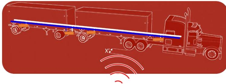
Our research indicates that J2497 (PLC4TRUCKS) receivers are susceptible to remote RF induced signals. This can be accomplished with a range of equipment costs for a range of distances from ~300 USD to ~10KUSD and up to 12ft. We have found that all 3 trailer ABS supplier's equipment are affected. Additionally, both tractor ABS controller supplier's equipment are also affected. We have found that some trailer configurations/types are more susceptible to RF induced J2497:
